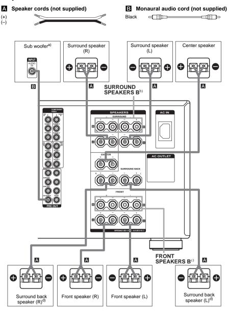
a) When you connect a sub woofer with an auto standby function, turn off the function when watching movies.
